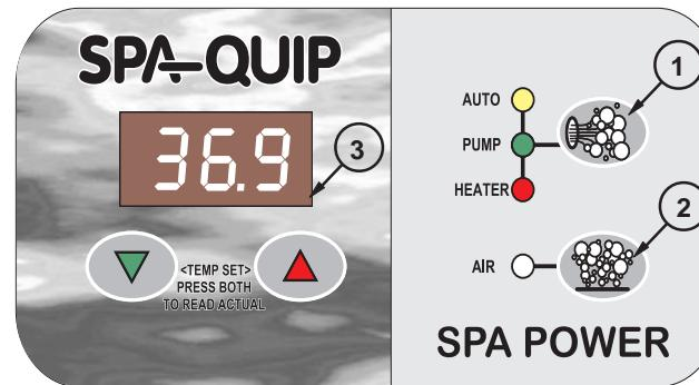
The Pump Mode button allows the user to switch the pump on or off as desired when using the pool. For safety the heater is always automatically controlled. Automatic operation is the default and the system returns to automatic mode by itself at a fixed time (90 minutes) after the user last pushed the pump mode button. Pushing the pump mode button then switches the pump on and terminates automatic mode. If the pump was already on in auto mode then it will stay on.
