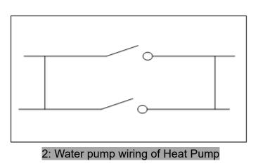
Note: The installer should connect 1 parallel with 2 (as above picture). To start the water pump, condition 1 or 2 is connected. To stop the water pump, both 1 and 2 should be disconnected.
