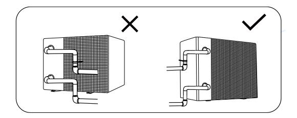
**DO NOT** install water pipes in such a way that they pass behind the heat pump's evaporator. In the case this cannot be avoided, cover the pipes with thermal insulation foam.
